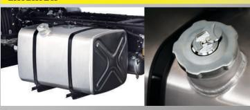
▲ Bigger and durable aluminium alloy fuel tank with lockable cap.
