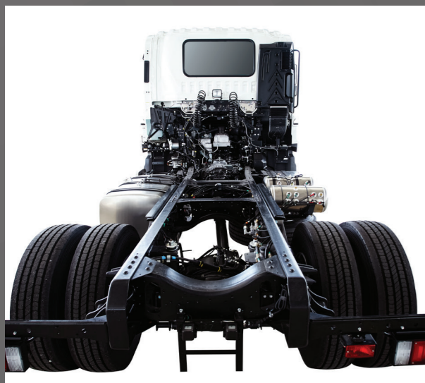
Double layer chassis frame.
