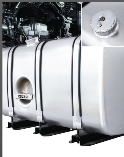
Bigger and durable aluminium alloy fuel tank with lockable cap.
