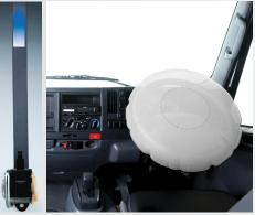
\*SRS airbag system and seat belt with pretensioner are activated in the Cabin Tilt Warning & Buzzer for event of a frontal collision, mitigating impact to the head and chest. \*Applicable for driver only.
